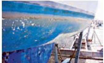
Paint blisters and lifts
