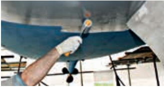
Apply Hempel's High Protect with roller
