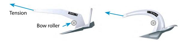
It is ideal to lash your anchor with rope when underway. The Rocna features a dedicated lashing point, and the tandem anchor attachment point may be used on both the Rocna and Vulcan. On the larger sizes we do not recommend that these holes be used for restraining pins, as a wave hitting the anchor at sea could bend and so jam the bar. Do not drill new holes in the anchor shank – this will weaken the shank and void the warranty.
