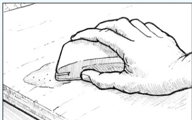
Figure 23 Sand cured fairing compound to desired contour.
