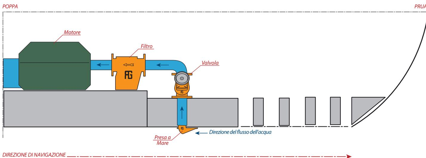
**Guidi System installation drawing (water inlet, non-stick valve, filter)**
