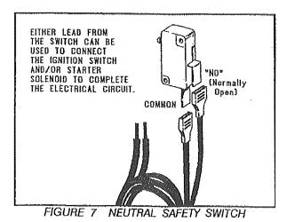
Connect the Neutral Safety Switch between the Ignition switch (start lead) and the starter solenoid,
