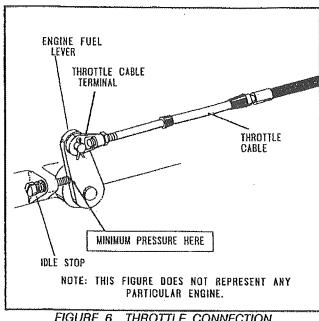
FIGURE 6 THROTTLE CONNECTION
