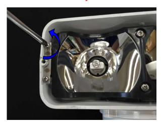
A-4. (Operations: Pull out power head and remove lamp and motor from the connection terminal. / Tools: None required.)
