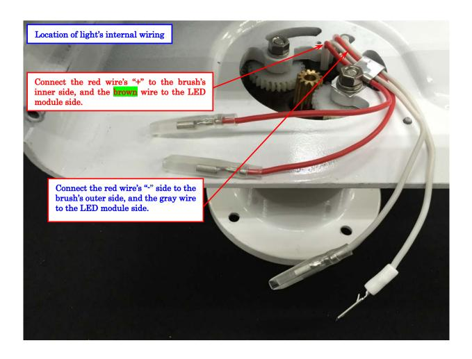
C-2. (Operation: Return LED powerhead to the lamp. / Tools: None required.)
