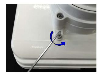
A-2. (Operations: Remove mounting screws (M4 × 2 locations) on frame. / Tool: ②)
