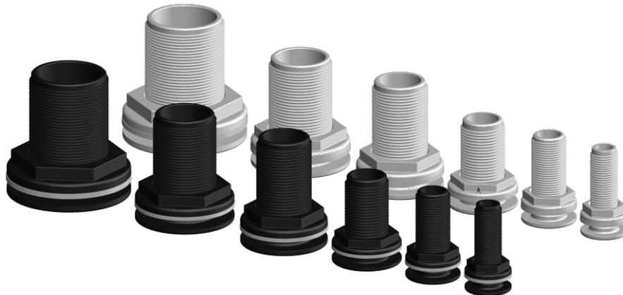
The Skin Fitting body and nut are moulded from glass fibre reinforced nylon composite. High strength, high-modulus glass fibres provide dramatic strength, stiffness, toughness and dimensional stability. These properties allow a significant weight reduction over metallic fittings.
