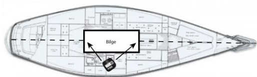
Figure 6 ME SENSE positioning of bilge sensor
