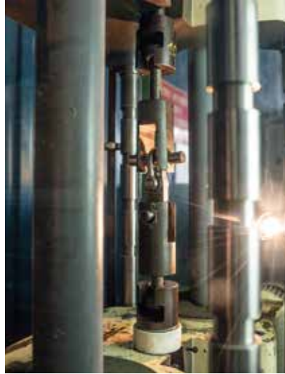
Test/traction bench for mechanical resistance
