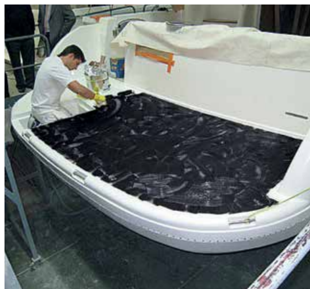
Fig. 52 Application of Sikaflex®-298
