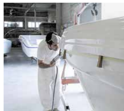
Fig. 102 Sealing with Sikaflex®-295 UV
