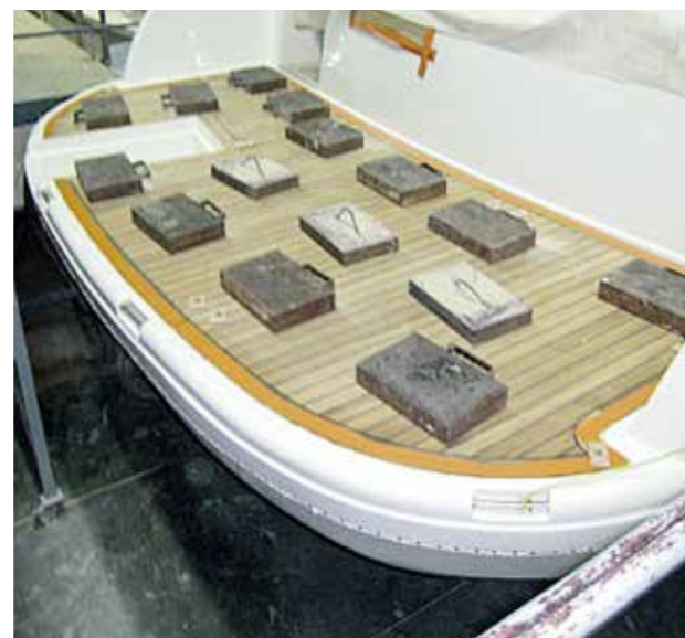
Fig. 53 Holding in place with weights
