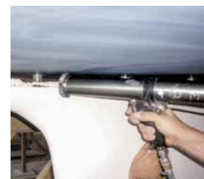
Fig. 106 The adhesive is applied
