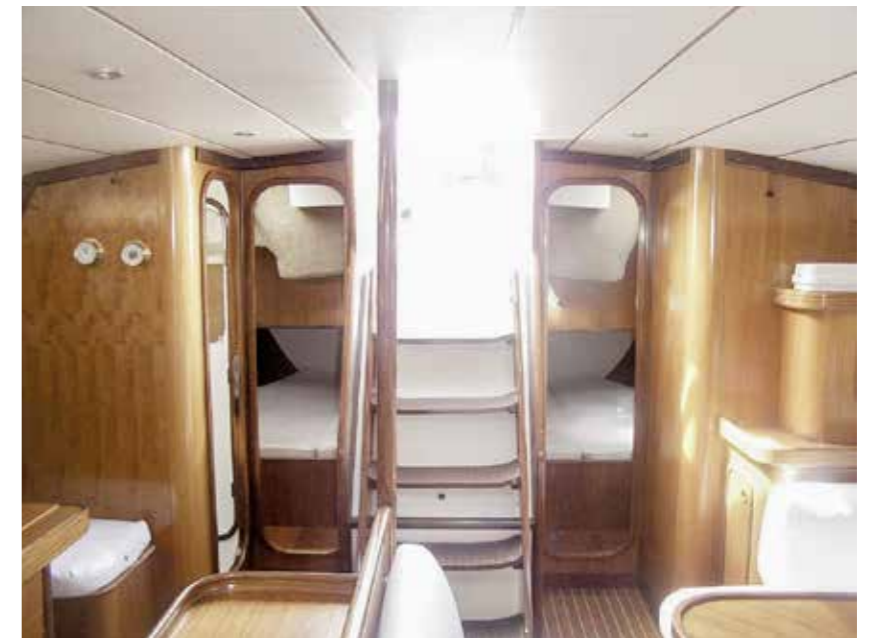
Fig. 94 High-quality lightweight panels finished in traditional high-gloss wood veneer and bonded using Sikaflex®-292i
