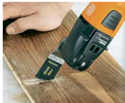
Fig. 74 Cutting planks with vibrating knife
