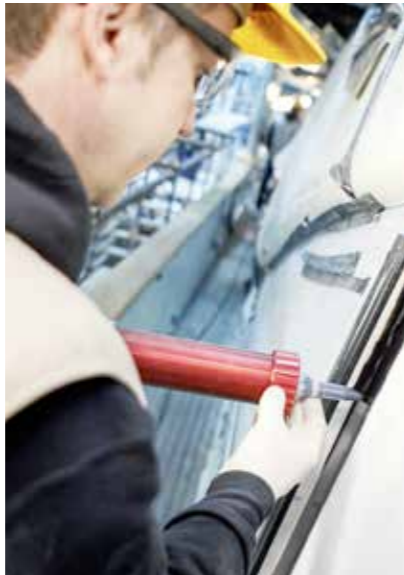
Fig. 100 Adhesive is applied to the window frame
