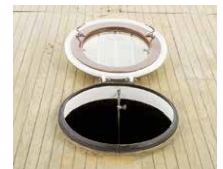
Fig. 84 A port-hatch, both bonded and sealed using Sikaflex®
