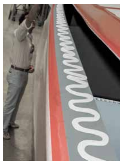
Fig. 103 Hull and deck are brought together
