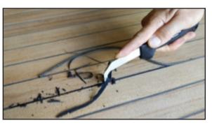
2. Reefing hook scrapes out caulk sealants once they have been freed using a razor knife. It leaves minimal material residue, so the seam can be easily sanded.
