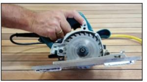
**4.** Note: A seam saw may be used especially for minimal seam depth requirements. Saw safety cap should be on before using. (Cap in photo removed only to show blade.)
