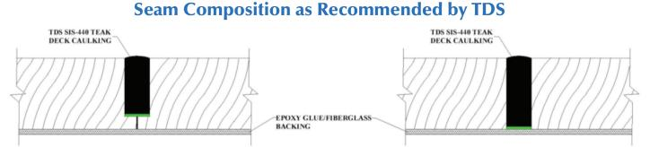
Use of polypropylene bond breaker tape in seams of 6mm and deeper. It aids to achieve 2-sided adhesion. The bottom of seam must be flat and square. The caulk seam should be able to move at the base of the seam, as the deck flexes and works.
