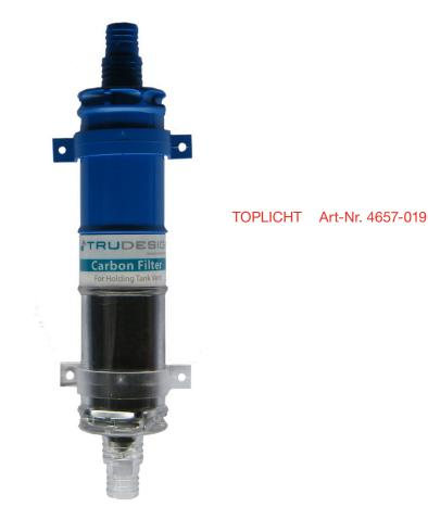
The Carbon Filter is not a substitute for good ventilation of the holding tank. It is designed to remove excess odour from a properly functioning holding tank. Holding tanks require good ventilation to ensure aerobic decomposition. Anaerobic decomposition due to lack of oxygen is the major cause of holding tank odour through  $H_2S$  production (rotten egg smell).
